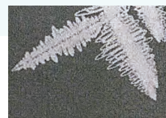
Dendritic growth is a fundamental process observed in the casting of metals. This image is of dendrites of succinonitrile grown in space during the first IDGE flight. 27
